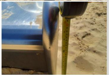
**Finding:** The height of the slide runout is in excess of 350mm and does not meet the requirements of BS EN 1176: levels Part 3
