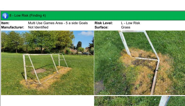
Finding: The goal frame has only been secured at one end Action: Refer to manufacturer recommendations and provide as required
