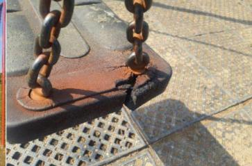
Finding: The seat has been severely damaged
