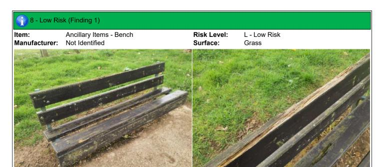
**Finding:** There are areas or parts of the timber on the structure that have rotted
