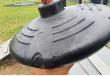
Finding: The cableway seat has been damaged
