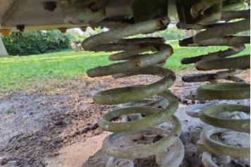
**Finding:** The paintwork on the spring has been damaged or **Action:** Treat any rusting components and repaint worn exposing the metal underneath which is rusting
