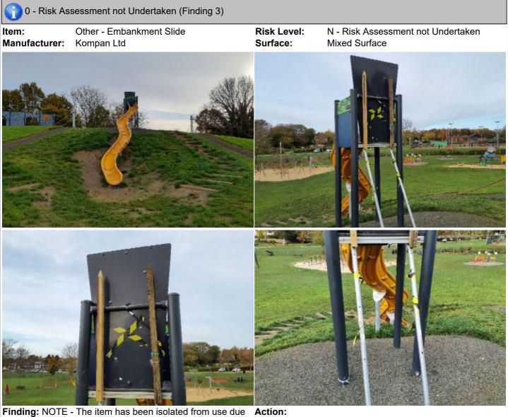
**Finding:** NOTE - The item has been isolated from use due **Actie** to accidents that have occurred. The access element has been removed and a full inspection could not be undertaken of the platform / starting area
