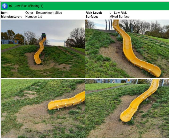
**Finding:** The grass has eroded within the impact area of the **Action:** Reinstate the grass or provide an all weather equipment and may not provide the necessary impact surface attenuating properties for the equipment fall height; the surface may also be slippery in wet weather
