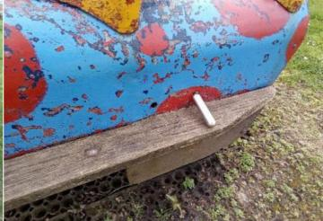
**Finding:** There is/are finger entrapment/s in the rocking horse frame and the item fails to meet the requirements of BS EN 1176 Part 1 4.2.7.6 Entrapment of fingers
