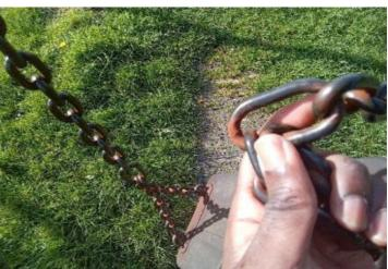
Finding: There is some notable evidence of connecting link Action: Monitor for any further deterioration and replace when 40% worn
