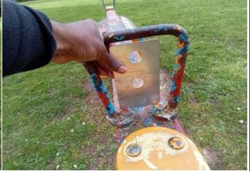
**Finding:** The item fails to meet the requirements of BS EN 1176 Part 1 4.2.7.2 for head and neck entrapment in the see saw handles
