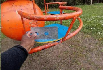
Finding: The item fails to meet the requirements of BS EN Action: Monitor - No remedial work recommended 1176 Part 1 4.2.7.2 for head and neck entrapment in the roundabout
