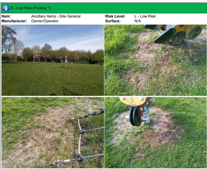
**Finding:** The grass mats are silted up, the soil is compacted **Action:** Reinstate as required and the area will become very slippery when the soil is wet.
