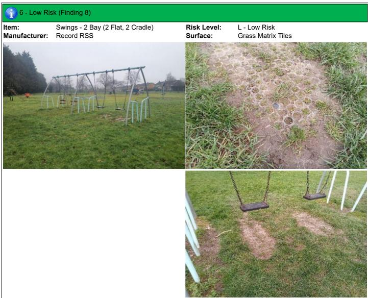
**Finding:** Fixing Pins have been installed in the impact areas **Action:** Remove pins from impact areas of the grass mats
